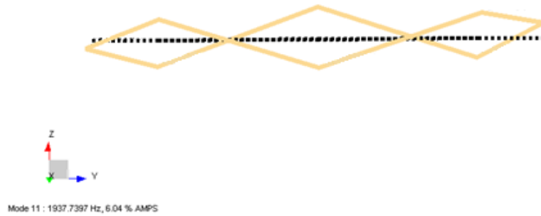
Figure 4.11 Third mode shape obtained from LMS Test Lab software for the Type-2 coil sample.
